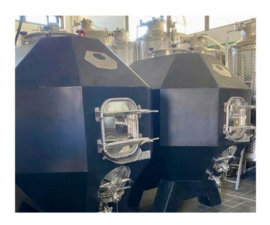
controlled oxygen transfer but also has excellent thermal properties. This excites us because it combines the best of both worlds: the oxygen permeability of wood (without imparting flavor) and the neutrality of stainless steel. It also enables gradual temperature adjustments during fermentation or maturation, avoiding the abrupt changes that can occur in stainless steel tanks—thus treating the wine more gently.
